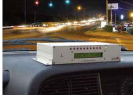
MPC555-based electronic control module, pictured on the vehicle dashboard. Photo courtesy of add2 Ltd.
